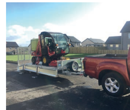
Can load pallets with forklift from the side using removable drop sides
